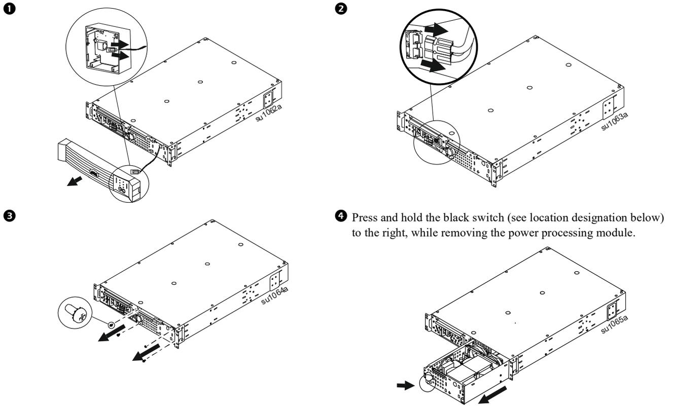
**Note:** Reverse steps 1-4 for installation of the new module.
