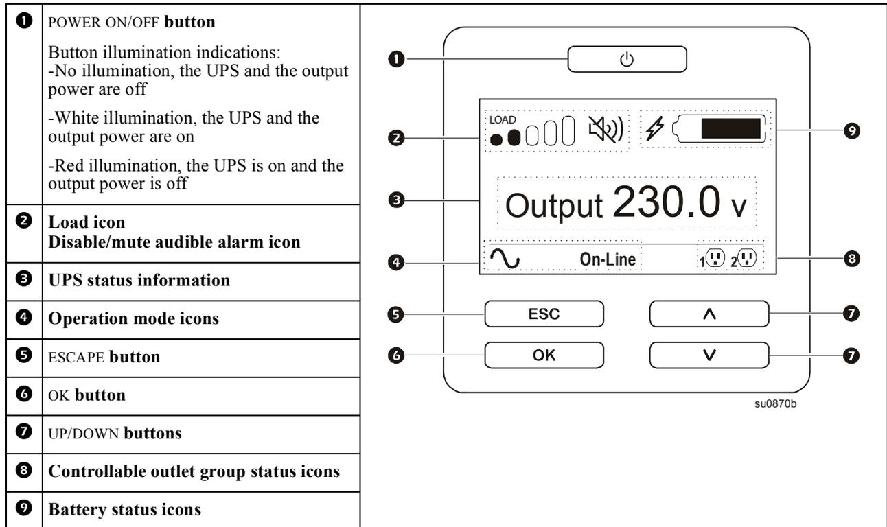
The icons on the LCD display interface screen may vary depending on the installed firmware version.
