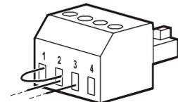
**Note:** Pin 1 is the power source for the EPO circuit, it provides a few milliamperes of 24 V power.
