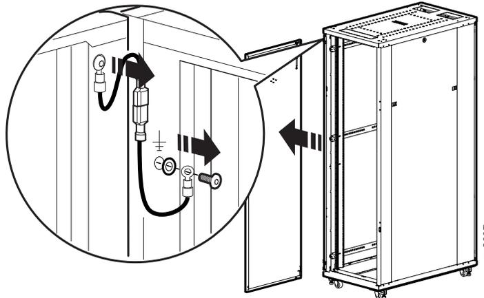
3. Rotate and reinstall the door to the opposite side. Remove any plastic hole plugs and reinstall the ground wire to the door and cabinet.
