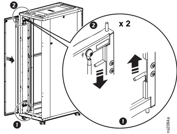
3. Connect the grounding wires.
