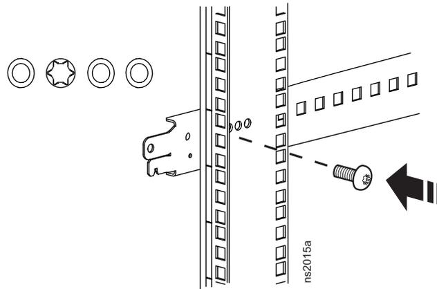
3. Perform the vertical mounting flange adjustment to the opposite side of the cabinet. Ensure that the same mounting position is used at the top, middle and bottom. Torque to 28 - 30 in-lb (3.2 - 3.4 N-m).
