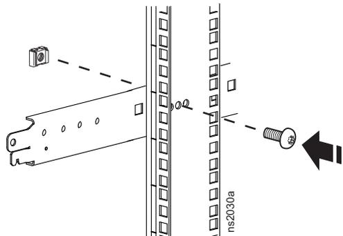
2. Move the mounting flange to the desired location and reinstall the T30 fastener at the top, middle and bottom to secure the vertical mounting flange.
