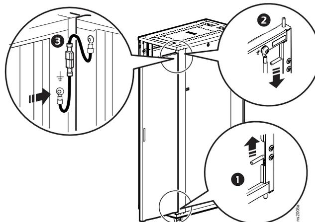
4. Remove and reinstall the latch and washer oriented as shown using a Torx T30/#2 Phillips wrench. The washer is rotated 90 degrees from its original orientation, and the latch is rotated 180 degrees.
