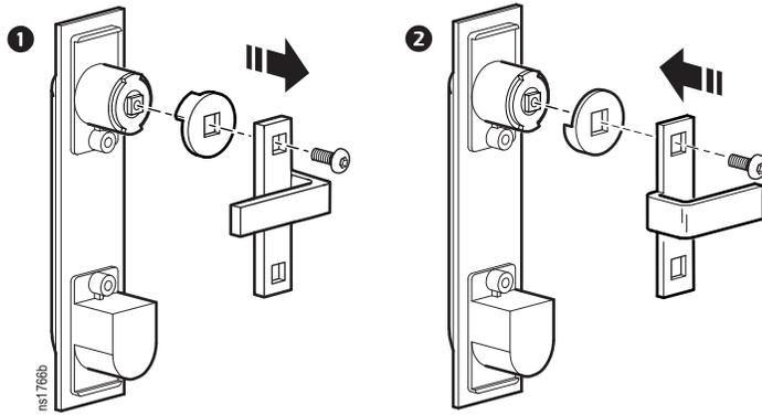
5. Reinstall the handle to the door. Torque the screws to 28 - 30 in-lb (3.2 - 3.4 N-m).
