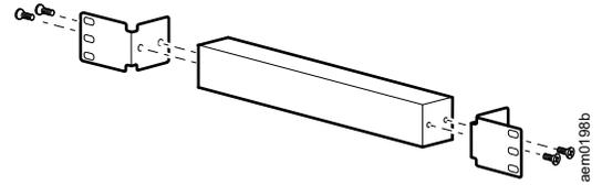
3. Secure the Rack Monitor 250 to the rack, using cage nuts and screws (not provided).
