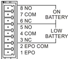
The relays are connected from the common (COM) to the normally closed (NC) pins. When the unit enters a low battery or on battery state, the appropriate relay will transition and connect the common (COM) to the normally open (NO) pin.
