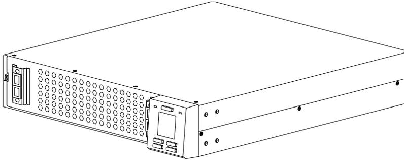
② Pull out the LCD display on the UPS.
