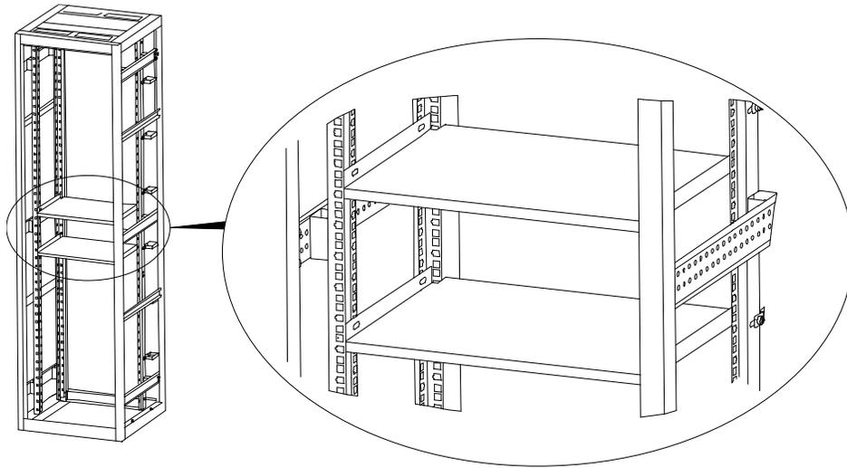
Follow the instructions below to secure and position battery pack into the 19 inch rack enclosure.
