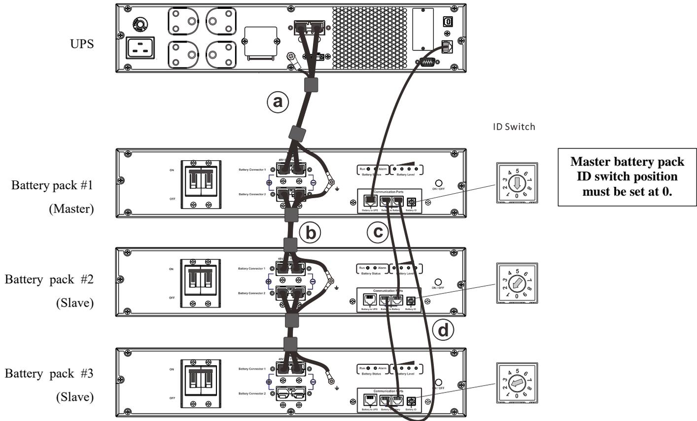
1. Connect one end of battery cable **a** to the battery connector terminals on the UPS and the other end to the CON 1 receptacle on the battery pack. Be sure to connect the ground wire securely.
