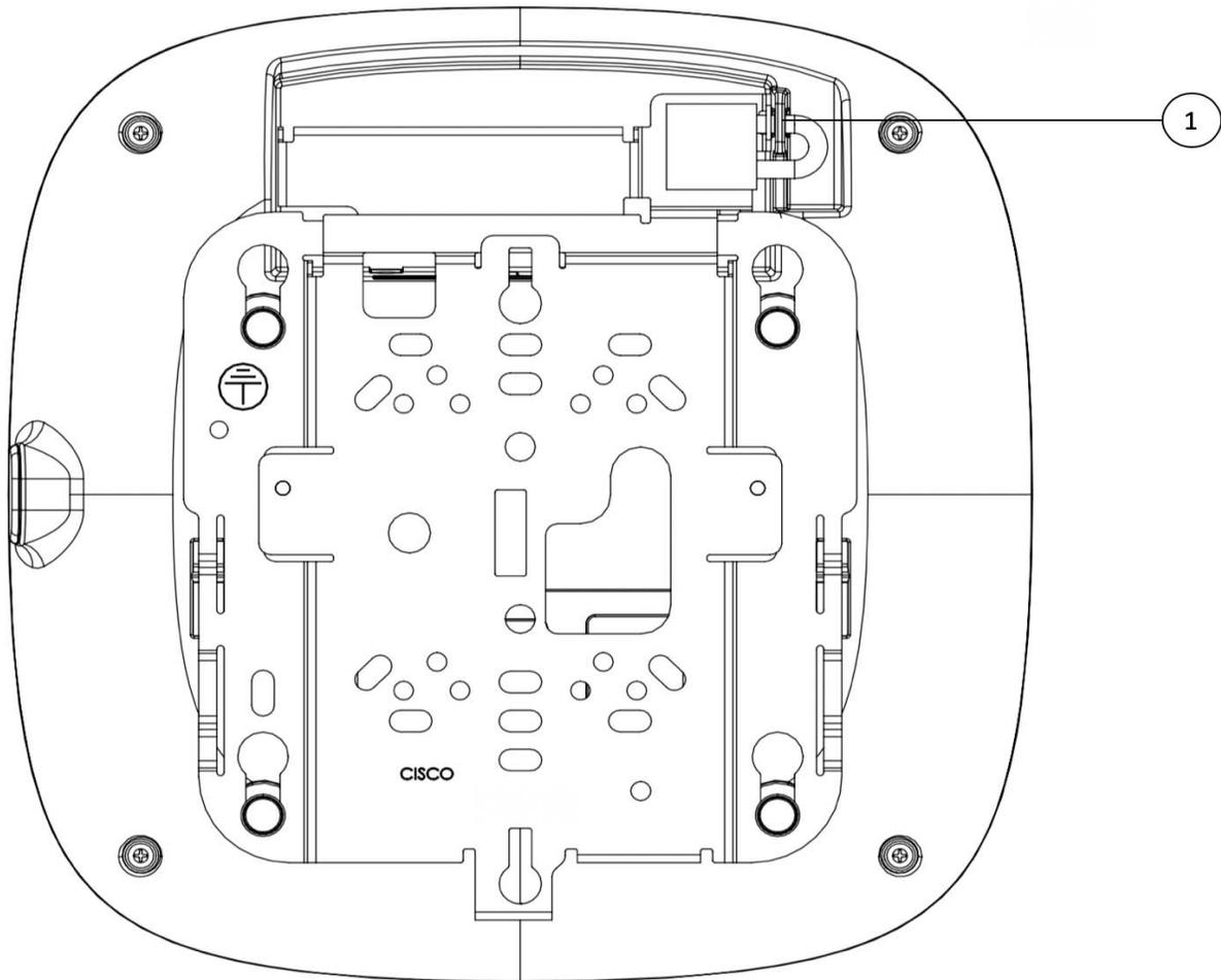
**1** Position of the hasps for the locks on the back of the 9120AXI model
