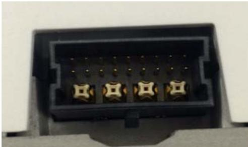
**Figure 12** AIR-CAB002-DART-R= DART Connector
