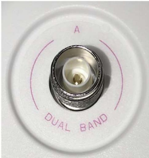
The remaining dual-band RP-TNC ports that do not support Self-Identifying Antennas can be differentiated by the standard orange color text around the connector. Self-Identifying Antennas can be used on any of the RP-TNC ports of the AP. However, only port A will read the antenna as a Self-Identifying Antenna.
