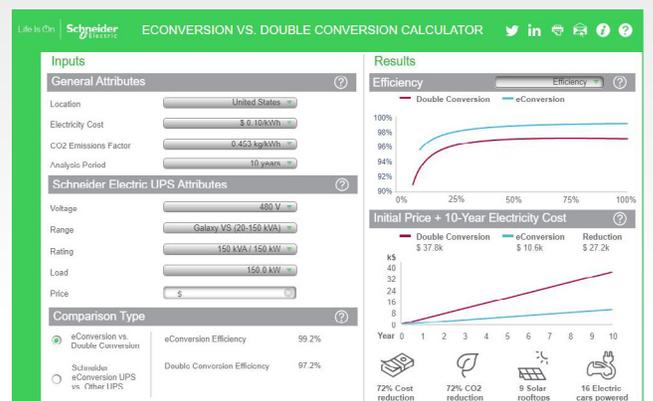
\*Model dependent; based on a market electricity price: \$0.15 /kWh. The annual electricity savings are calculated by comparing the UPS efficiency in eConversion mode vs. double conversion mode.
