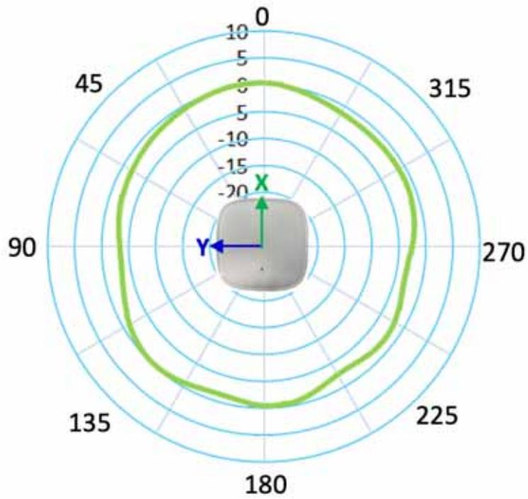
Figure 6 C9105AXI and C9105AXIT — BLE Antenna — Elevation
