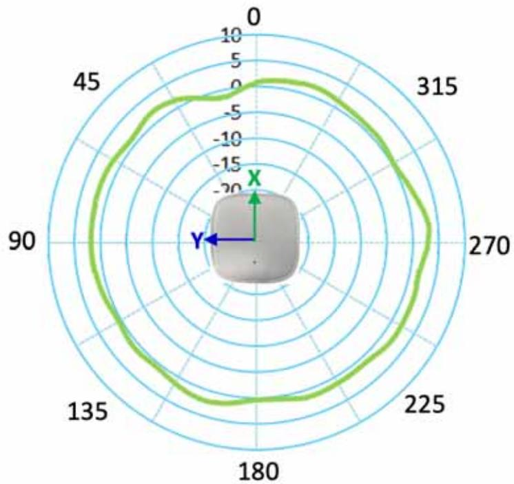
Figure 4 C9105AXI and C9105AXIT — Dual-band Antenna (5 GHz) — Elevation
