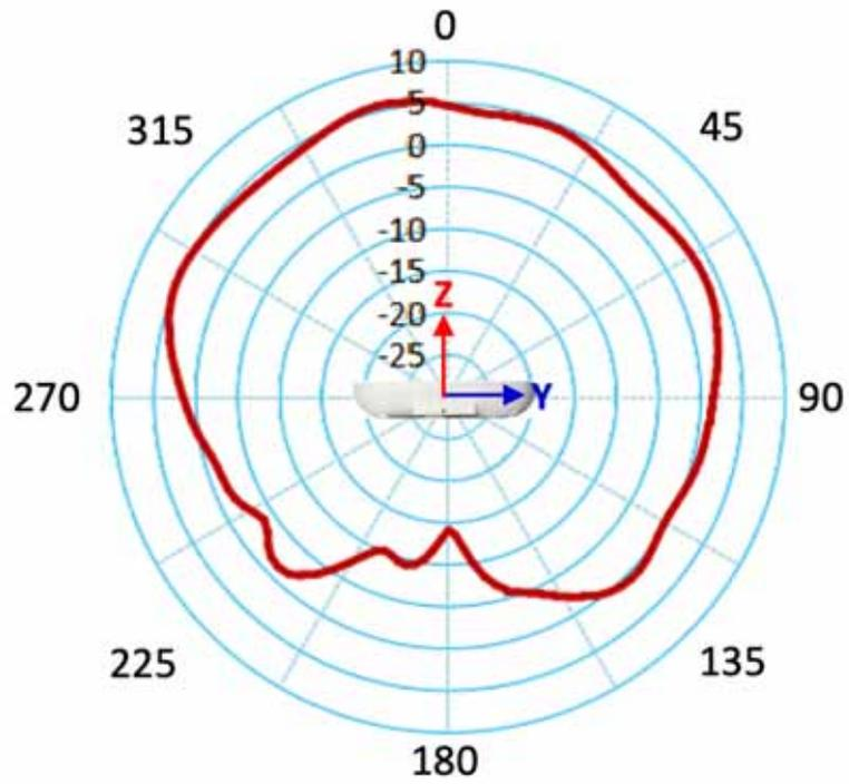
Figure 5 C9105AXI and C9105AXIT — BLE Antenna — Azimuth
