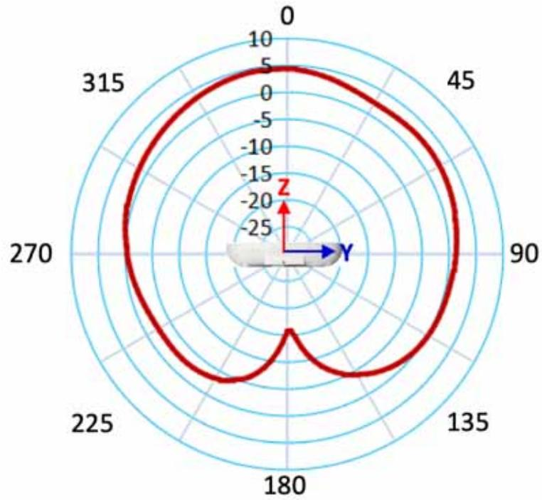
Figure 3 C9105AXI and C9105AXIT — Dual-band Antenna (5 GHz) — Azimuth
